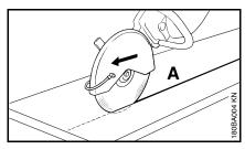
Work along the cutting line. If corrections are necessary, always reposition the cutting wheel, taking care to ensure that it is not wedged. The cutting depth per pass should not exceed 5 to 6 cm (2" to 2 1/2"). Thicker material must be cut in several passes.
