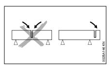
Be alert to potential movement of the workpiece or anything else that could cause the cut to close and pinch the wheel. In order to reduce the risk of
