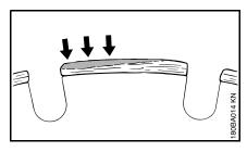
Built-up edges are identified by a pale grey deposit on the top of the diamond segments that clogs and blunts the segments.
