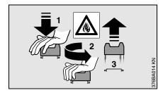
Never use a tool to open or close the bayonet fuel filler cap, as this could damage the cap and cause fuel to leak out.
