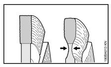
Undercutting is a wearing away of the steel core at or just below the diamond segments. When cutting road surfaces, do not cut through into the more abrasive ballast (gravel, crushed rock) below, as indicated by a light colored dust. This can cause excessive undercutting, resulting in wheel breakage and/or thrown segments.
