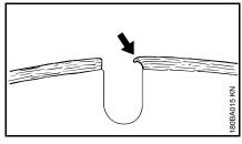
If you continue to use a cutting wheel with blunt segments, the segments may soften as a result of excessive heat built up. The wheel core will also overheat and lose its mechanical strength. This can lead to considerable stress, as clearly indicated by stress cracks and/or a wobbling movement of the cutting wheel.
