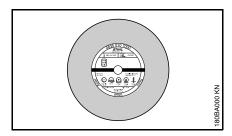
Economic benefit is improved and premature wear can be avoided by choosing and using the correct composite resin cutting wheel. The short name (e.g. "asphalt", "concrete")
