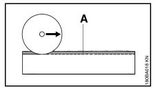
Cut a guiding groove (A) along the marked line.
