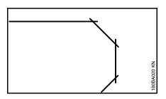
Curves must be cut in several straight passes, taking care to ensure that the cutting wheel does not become wedged.
