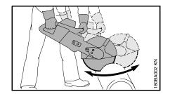
Thick-walled workpieces should be cut with a uniform swinging movement, back and forth.
