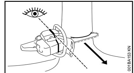
When making the felling notch, use the gunning sight on the shroud and housing to check the desired direction of fall:
