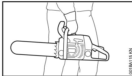
It may be carried only in a horizontal position. Grip the front handle in a manner that the machine is balanced
