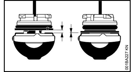
Left: Base of cap in closed position (with open space)
