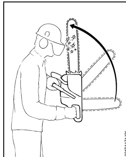
All STIHL chain saws are equipped with a Quickstop chain brake which can be activated by inertia. If the forces of an occurring kickback are sufficiently high,
