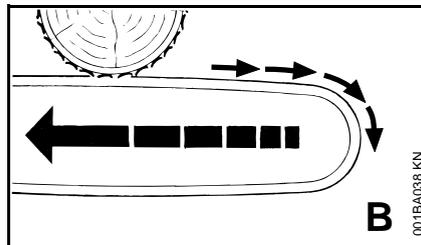
Pushback occurs when the chain on the top of the bar is suddenly stopped when it is pinched, caught or encounters a foreign object in the wood. The reaction of the chain may drive the saw rapidly straight back toward the operator and may cause loss of saw control. Pushback frequently occurs when the top of the bar is used for cutting.
