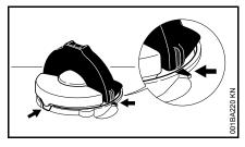
To do this with this STIHL cap, raise the grip on the top of the cap until it is upright at a 90° angle. Insert the cap in the fuel tank opening with the raised positioning marks on the grip of the cap and on the fuel tank opening lining up. Using the grip, press the cap down firmly while turning it clockwise as far as it will go (approx. 1/4 turn).
