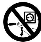
Never direct the high-pressure jet or water hose against electrical equipment, connections and power cords – **danger of short-circuiting!**
