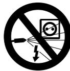
Never direct the high-pressure jet or water hose against electrical equipment, connections and power cables – **danger of short-circuiting!**
