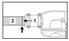
Push the gearbox (1) onto the shaft (2) as far as stop – turn the gearbox back and forth until the square end of the shaft engages
