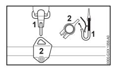
Attach the carabiner (1) to the carrying ring (2) on the shaft.
