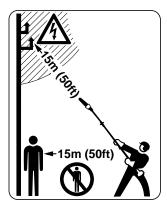
Do not allow other persons within a radius of 15 m of your own position due to falling branches and ejected wood particles – **Risk of injury!** This distance must also be maintained in relation to objects (vehicles, window panes) – **risk of property damage!**
