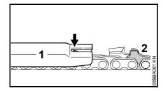
Place a filing gauge (1) that matches the chain pitch on the chain and press it against the cutter
