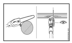
To avoid pinching the bar in the cut, position the cutting attachment with the hook against the branch and then perform the cross-cut from the top
