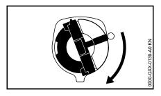
Hold the fuel cap down and twist it clockwise until it engages
