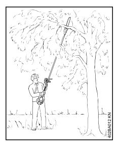
The shaft should always be held at an angle of 60° or less.
