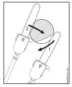
To avoid tearing the bark on thick branches, always start by performing a
