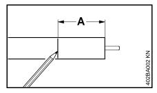
Apply a mark to the shaft at distance
