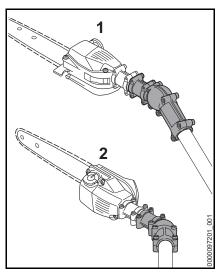
The angle drive keeps the cutting attachment at an angle of 30° to the shaft.
