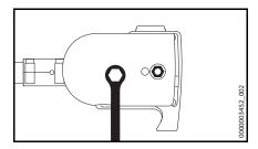
Unscrew the nut and remove the cover
