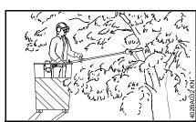
The machine's long reach enables cutting to be performed next to the trunk without the risk of the lift bucket damaging other branches. The tool angle in this case depends on the position of the branch.
