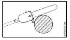
When performing the separating cut, position the bar against the branch near the hook. This will prevent the power tool from making jolting movements when you start the separating cut.
