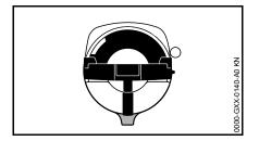
Then the markings on fuel cap and oil tank will align
