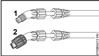
A hollow cone nozzle (1) or fan jet nozzle (2) can be fitted to suit requirements.
