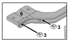
• Fit the square nuts (3) in the barrier bar (6); the holes must line up.
