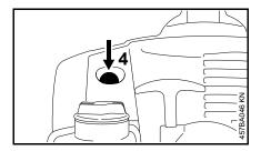
Press the manual fuel pump bulb (4) at least five times – even if the bulb is filled with fuel.
