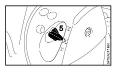
Press in the choke lever (5) and turn it to z at the same time. Also use this setting if the engine has been running but is still cold.
