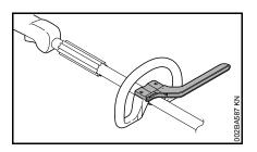
A barrier bar may have to be mounted to suit the cutting attachment you intend to use – see "Approved Combinations of Cutting Attachment, Deflector, Handle and Harness".
