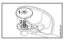
• Slip the thrust plate (1) over the shaft (2).
