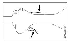
Press down the throttle trigger lockout and open the throttle – the choke lever moves to the run position I. After a cold start, warm up the engine by opening the throttle several times.
