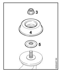
The nut (3), rider plate (4) and thrust washer (5) are required to secure some mowing heads.
