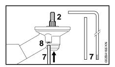
The output shaft (2) must be blocked with the stop pin (7) or screwdriver (7) to mount or remove cutting tools. These parts come standard with the machine or are available as special accessories.
