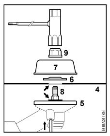
• Place the cutting attachment (4) on the thrust plate (5).
