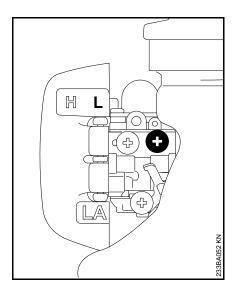
Determine the standard setting as follows: Turn the low speed screw (L) carefully clockwise as far as stop, then turn it counterclockwise.
