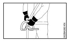
On models with a loop handle and barrier bar, left hand on loop handle, right hand on control handle, even if you are left-handed.
