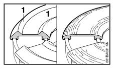
If the raised moldings (1) on the base of the attachment are worn as shown in the illustration (above right), do not continue using the mowing head. Install a new one. There is otherwise a risk of injury from thrown parts of the head.
