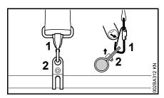
Press down the bar on the carabiner (1) and pull the carrying ring (2) out of the carabiner.
