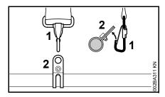
• Attach the carabiner (1) to the carrying ring (2) on the drive tube.
