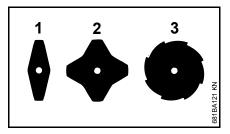
The **skirt and line limiting blade** are not required on the deflector for grass cutting blades 230-2 (1), 230-4 (2) or 230-8 (3) – see "Mounting the Deflector".
