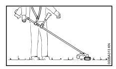
Mowing heads and grass cutting blades should just touch the ground.
