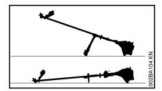
Lay your brushcutter on its back so that the cutting attachment mounting face is facing up.
