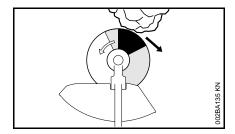
The risk of kickout is greatest when the black area of the rotating blade comes into contact with a solid object.
