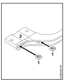
• Fit the square nuts (1) in the barrier bar (2); the holes must line up.
