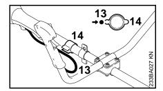
Press throttle cable (13) into the throttle cable support (14)
