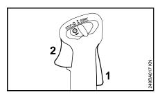
Press down the trigger interlock (1) and squeeze the throttle trigger (2) (full throttle) – this sets the throttle cable correctly.
