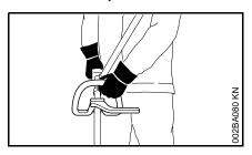
On units with a loop handle and barrier bar, left hand on loop handle, right hand on control handle, even if you are lefthanded.
