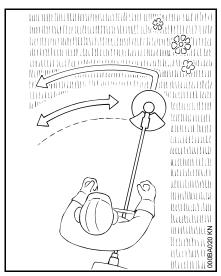
Use for cutting grass and weeds only. Sweep the brushcutter in an arc like a scythe.
