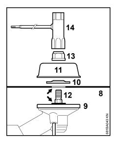
Lay your brushcutter on its back with the cutting tool mounting face pointing up:
