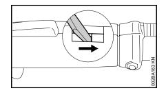
Use a suitable tool to push the slide to the bottom of the slot (see illustration).
