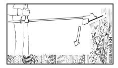
To cut wild growth and scrub, lower the **brush knife down** onto the growth to achieve shredding effect – do not use the cutting tool above waist height.
