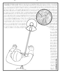
Nylon line achieves a soft cut for edging and trimming around fence posts, trees, etc. – less risk of damaging tree bark.
