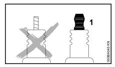
If the spark plug comes with a detachable adapter nut (1), screw it on firmly.
