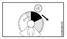
The risk of kickout is highest in the black area area of the blade: Do not use this area of the circular saw blade for cutting.
