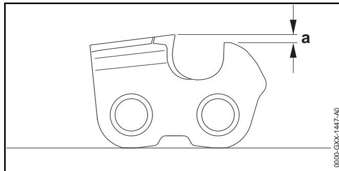
The depth gauge determines the depth to which the cutter penetrates the wood and thus the chip thickness.
