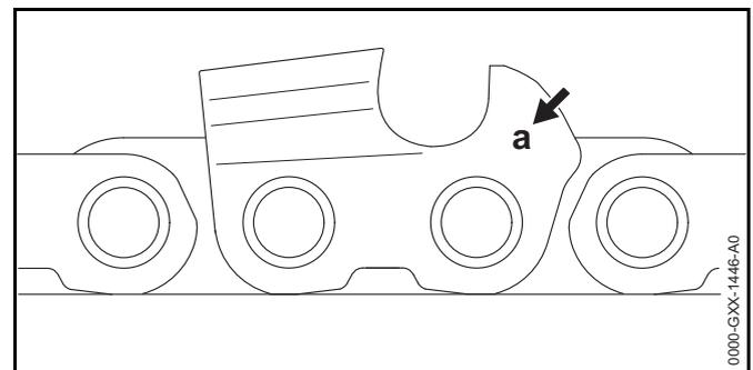
The chain pitch marking (a) is embossed in the area of the depth gauge of each cutter.
