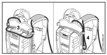
The length of the connecting cable can be adjusted by making a loop on the backplate (3) or at one side (4).
