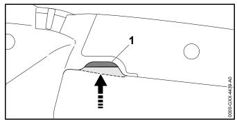
Override the trigger's (1) end position and hold it there. The LEDs flash in sequence. The boost function is activated.
