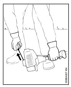
Place the machine on the ground – it must rest securely on the machine support and the gearbox.
