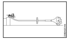
Place the edger so that the blade mounting (1) faces upwards
