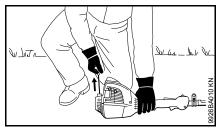
Place the machine on the ground in a secure position
