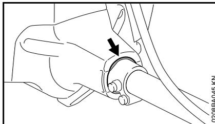
A vibration-absorbing rubber element is installed between the powerhead and the shaft. Have it checked in the event of noticeable wear or constantly increased vibration.
