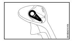
Move the setting lever to 0 – the engine stops – the setting lever springs back to the on position.
