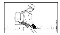
The unit is carried as a backpack. Hold and control the blower tube with your right hand on the control handle.
