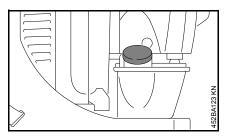
Before fueling, clean the filler cap and the area around it to ensure that no dirt falls into the tank
