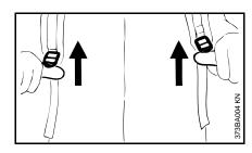
Lift the tabs of the sliding adjusters.
