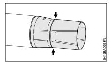
The front end of the nozzle wears away due to abrasive ground contact during operation. The nozzle is subject to normal wear and tear and must be replaced when the wear mark is reached.
