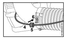
• Engage the throttle cable (4) with sleeve (5) in the retainer (6).
