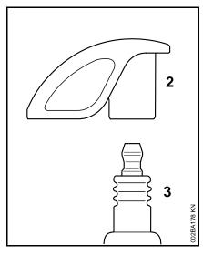
Screw the spark plug (3) into the cylinder and fit the boot (2) (press it down firmly).
