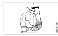
• Secure the blower tube to the handle on the backplate.
