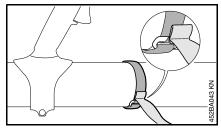
Secure the velcro strip to the blower tube – pull the flap through the buckle.
