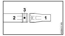
Push the nozzle (1) onto the blower tube (2) and engage it on the lugs (3).
