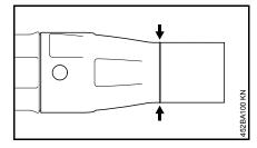
The front end of the nozzle is worn by ground contact during operation. Replace the nozzle when it has worn as far as the wear mark.
