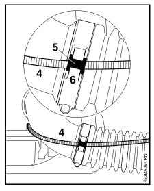
Engage the throttle cable (4) with sleeve (5) in the retainer (6).
