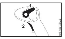
• Push the setting lever (1) upwards. The throttle trigger (2) is in the full throttle position.
