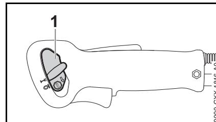
The slide control (1) is in the normal run position I.
