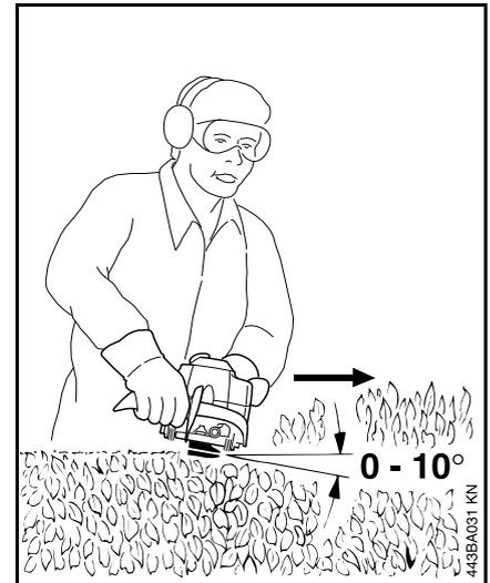
Hold the cutter bar at an angle of 0° to 10° as you swing the hedge trimmer horizontally.
