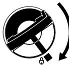
Place the clip lock fuel cap (bayonet-type) in position, turn it as far as it will and fold the clip lock down.
