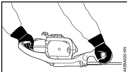
Left hand on the control handle, right hand on the cutterbar handle. Wrap your fingers and thumbs around the handles.
