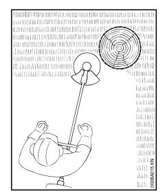
Nylon line achieves a soft cut for edging and trimming around trees, fence posts, etc. – less risk of damaging tree bark.
