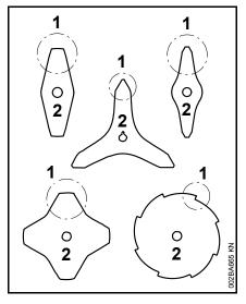
Resharpen the teeth (1) uniformly – do not alter the contour of the parent blade (2) in any way.
