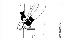
On models with a loop handle and barrier bar, left hand on loop handle, right hand on control handle, even if you are left-handed.
