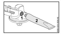
Check grease level after every 25 hours of operation and re-lubricate if necessary.
