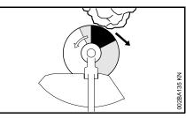
The **risk of kickout is greatest** when the **black area** of the rotating cutting attachment comes into contact with a solid object.
