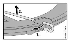
Disconnect wire rod from the transport guard.
