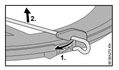
Disconnect wire rod from the transport guard.
