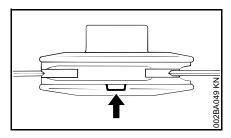
If one of the wear limit marks on the PolyCut mowing head is worn through (arrow): Do not continue using the mowing head. Install a new one. There is otherwise a **risk of injury** from thrown parts of the head.
