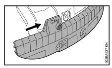
Slide the lower guide slot of the skirt onto the deflector – it must snap into position.
