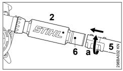
Push nozzle (5) in position (a) onto the blower tube (2) as far as lug (6) and rotate in direction of arrow to lock in position.
