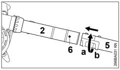
Push nozzle (5) onto blower tube (2) as far as lug (6), position (a) (long) or position (b) (short), and rotate nozzle in direction of arrow to lock in position.
