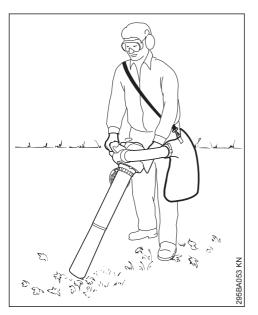
The vacuum attachment is designed for twohanded operation. Hold and operate the unit with your right hand on the control handle and your left hand on the assist handle.
