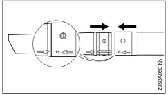
Line up the arrows on the suction tube and extension tube. Push together and lock in position.
