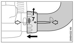
Push the union nut (7) over the fan housing stub as far as stop. Rotate the union nut (7) in direction of arrow until symbol is in line with the arrows – union nut snaps audibly into position.
