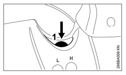
Press the manual fuel pump bulb (1) at least five times – even if the bulb is filled with fuel.
