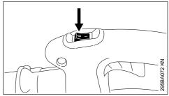
Move the stop switch to 0 – the engine stops – the stop switch springs back to the on position. English
