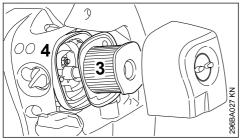
Take the air filter (3) out of the filter housing (4).
