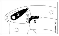
The setting lever (2) allows the throttle trigger (3) to be locked in any required position during operation.
