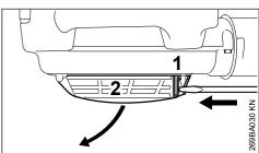
Insert screwdriver in the tab (1) and press down to disengage the intake screen (2) and then open the intake screen.
