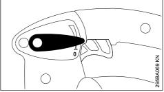
To start, move the setting lever to the run position I
