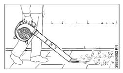
The blower is designed for one-handed operation. The operator must carry the blower with his right hand on the control handle.
