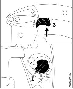
Blip the throttle trigger (3) – the choke knob moves to the run position I – the engine returns to idle speed.
