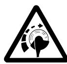
The cutting attachment continues to rotate for a short period after the throttle trigger is released (flywheel effect).
