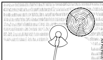
Mowing heads are to be used only on trimmers / brushcutters equipped with a line-limiting blade in the deflector in order to keep the line at the proper length (see "Main Parts" chapter in your instruction manual).
