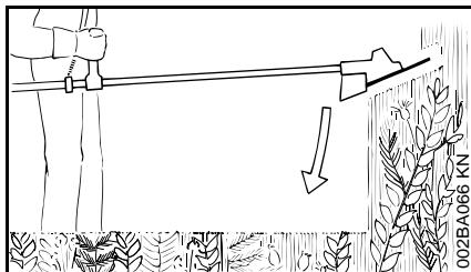
To cut wild growth and scrub, lower the rotating brush knife down onto the growth to achieve a chopping effect – but keep the tool below waist height at all times.
