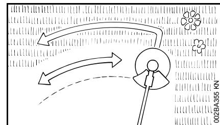
All kinds of grass and weeds can be easily cut with the grass cutting blade. The power tool is swept in an arc similar to a scythe.
