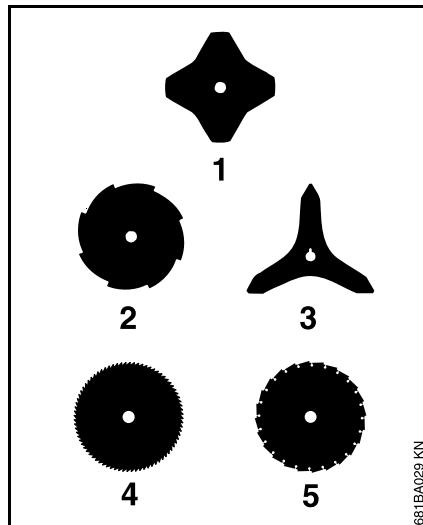
The **skirt and line limiting blade** are not required on the deflector for grass cutting blades 230-4 (1), 230-8 (2) or the brush knife (3) – see "Mounting the Deflector".
