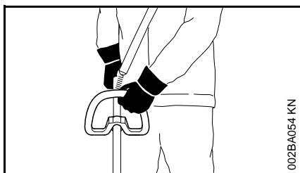
Always hold the unit firmly with both hands on the handles while you are working. Wrap your fingers and thumbs around the handles, keeping the handles cradled between your thumb and forefinger. Keep your hands in this position to have your power tool under control at all times. Make sure your trimmer handles and grips are in good condition and free of moisture, pitch, oil, fuel mix or grease.
