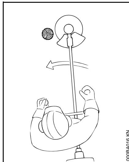
Circular saw blades are suitable for thinning brush and cutting small trees up to a diameter of 4 cm (1 1/2 in.). Do not attempt to cut trees with larger diameters, since the blade may catch or jerk the trimmer / brushcutter forward. This may cause damage to the blade or loss of control of the power tool and result in serious injury. Use a chain saw for such work.
