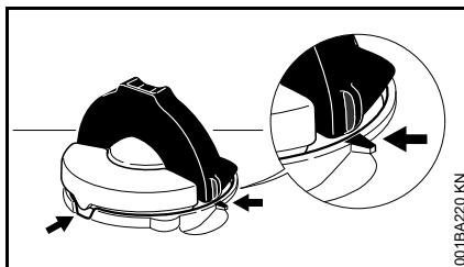
To do this with this STIHL cap, raise the grip on the top of the cap until it is upright at a 90° angle. Insert the cap in the fuel tank opening with the raised positioning
