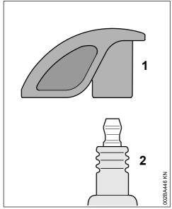
► Screw the spark plug (2) into the cylinder and fit the boot (1) (press it down firmly).
