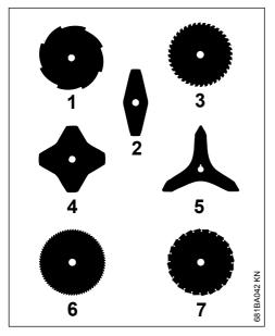
Cutting attachments 2, 4 and 5 may be mounted either way round – they must be turned over regularly to help avoid one-sided wear.
