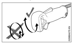
**Do not** rotate the control handle between unpacking and mounting it on the handlebar; see also chapter on "Adjusting the Throttle Cable".
