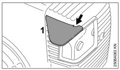
► Make sure the spacer (1) locates properly on the shroud (arrow)
