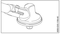
If the gearbox has no screw plug: gearbox is maintenance-free and requires no re-lubrication.
