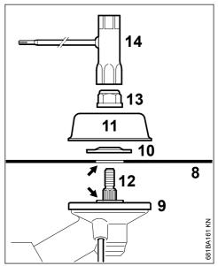
► Place the cutting attachment (8) on the thrust plate (9).
