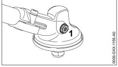
If the gearbox has a screw plug (1): Check grease level after every 25 hours of operation and re-lubricate if necessary.
