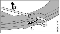
Disconnect wire rod from the transport guard.
