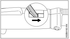
Use a suitable tool to push the slide to the end of the slot (see illustration).
