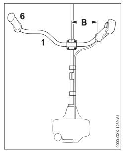
Place handlebar (1) in the handlebar support so that the distance (B) is not more than 15 cm (6 in) – the rubber handle (6) must be
