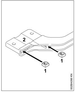
► Fit the square nuts (1) in the barrier bar (2); the holes must line up.
