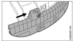
► Slide the lower guide slot of the skirt onto the deflector – it must snap into position.
