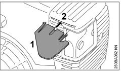
► Push the spacer (1) into the opening (2) in the shroud until it engages
