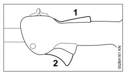
Press down the trigger lockout (1) and squeeze the throttle trigger (2) (full throttle position) – this sets the throttle cable correctly.
