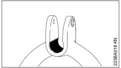
Place the friction liner in the loop handle.
