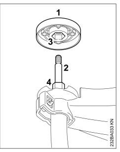
The thrust plate (1) is shipped with the Duro-Cut 5-2 and PolyCut 6-3. It is only required for these mowing heads.
