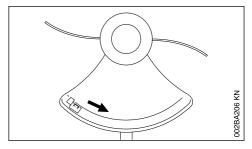
An arrow shows the direction of rotation of the cutting attachments.
