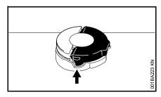
The lug on the bracket must engage entirely in the recess (arrow)
