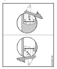
Perform this felling cut when the tree diameter is greater than the cutting length of the chainsaw.
