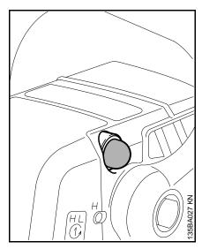
Press the manual fuel pump bulb at least five times – even if the bulb is already filled with fuel.
