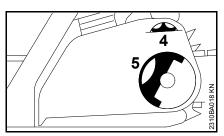
When fitting the chain sprocket cover, the teeth of the adjusting wheel and the tensioning gear must mesh; if necessary,
