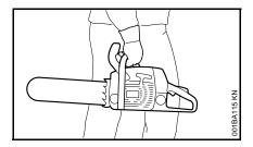
Always carry the chain saw by the handle – with the hot muffler away from your body, the guide bar must point to the rear. Avoid touching hot parts of the machine, especially the surface of the muffler – risk of burns!
