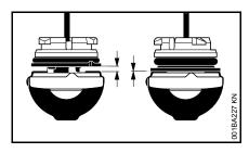
left: Base of filler cap twisted right: Base of filler cap correctly positioned
