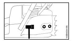
• Unscrew the nut and remove the chain sprocket cover.
