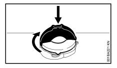
Hold the filler cap down and turn it clockwise until it engages
