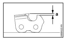
The depth gauge determines the depth to which the cutter penetrates the wood and thus the chip thickness. **a** Required distance between depth gauge and cutting edge
