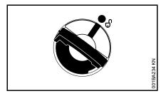
Markings on filler cap and fuel tank must align
