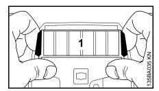
Place fingers behind the air filter (1), press thumbs against the housing and swing the filter in direction of rear handle.
