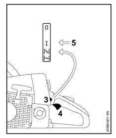
Press down trigger lockout and the blip the throttle trigger (4) – the Master Control lever (3) moves to the run position (I) and the engine settles down to idling speed.
