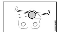
Guide the file: horizontally (at a right angle to the side surface of the guide bar) in accordance with the specified angle – according to the markings on the file holder – rest the file holder on the tooth head and the depth gauge
