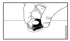
Grip the filler cap – if the filler cap cannot be moved or removed, then it is closed properly
