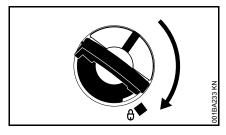
Hold the filler cap down and turn it clockwise until it engages
