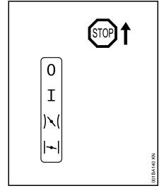
**Stop 0** – engine off – the ignition is switched off
