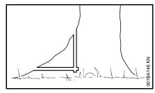
Remove largest buttresses: first the largest buttress – saw first vertically, then horizontally – only if the tree is in sound condition
