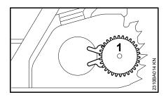
Remove and reverse tensioning gear (1)
