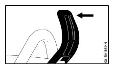
Pull the hand guard towards the front handle until there is an audible click – the chain brake is disengaged.
