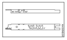
STIHL filing gauge (special accessory, see table "Sharpening tools") – a universal tool for checking sharpening and side plate angles, depth gauge setting, and tooth length, as well as cleaning grooves and oil inlet holes.
