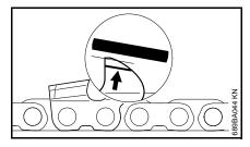
Afterwards, dress the leading edge of the depth gauge parallel to the service mark (see arrow) – when doing this, be careful not to further lower the highest point of the depth gauge
