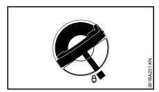
Then the markings on filler cap and fuel tank will align
