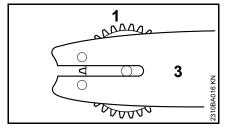
Position tensioning gear (1) and guide bar (3) relative to one another
