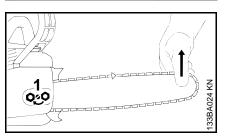
Retensioning during cutting work:
