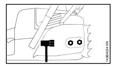
Unscrew the nuts and take off the chain sprocket cover.
