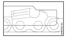
Lay the file gauge on the saw chain
